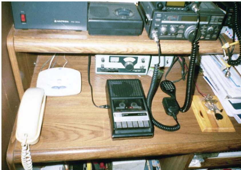
This is really all you need to record calls involving multiple radios; the recorder's built-in mic will pick up everything you say and hear, except the other side of telephone conversations. (Photo by the author.)
